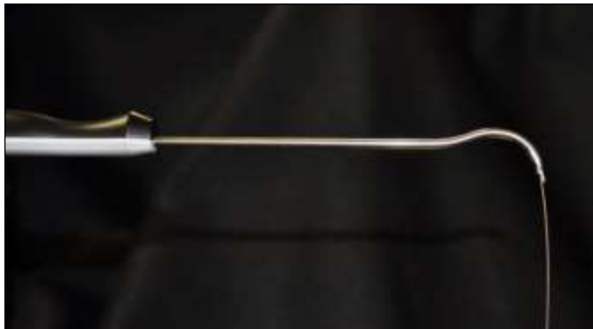
Fig 3.: Roll the Probe Handle until It is parallel with the floor.
