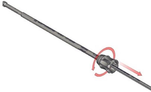
4. Gently rotate and wriggle the Outer Sleeve to align with the Inner Shaft's keyway. Pull backwards again to slide Outer Sleeve off the shaft.
